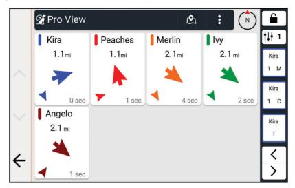
You can use the pro view feature to view the direction and distance to your dog and any paired devices. The pro view feature also shows the dog's status, such as running or on point (*Dog Status Icons*, page 15). The color of each pointer corresponds to the color of the track on the map.
